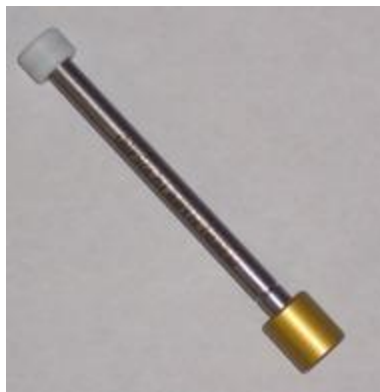
Figure 2-1: Photo of passive adsorbent sampler tube. Teflon cap (white) on one end and the diffusion cap (gold) on the opposite end.
