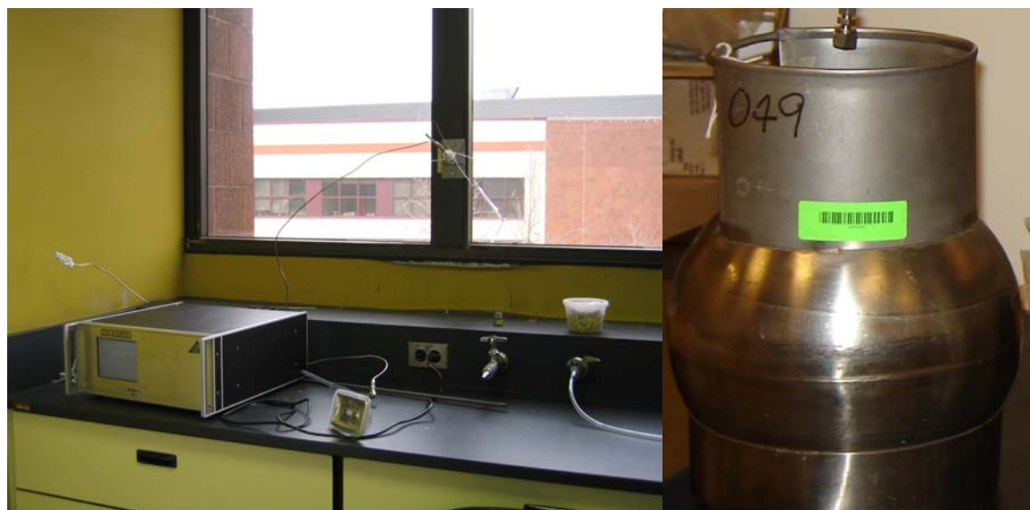
VOC Sampler at M Site: ATEC 2200; and a canister.
