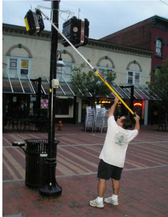
Figure 2. Hoisting Passive 3L and 6L Canister Samplers from Pole Bracket at Church St. Site
