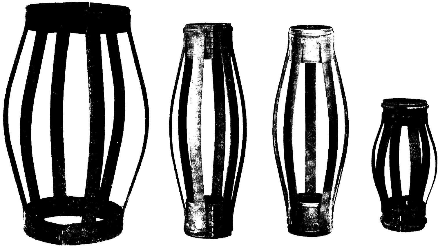
FIGURE 7-10. TYPES OF CASING CENTRALIZERS (SMITH, 1976).
