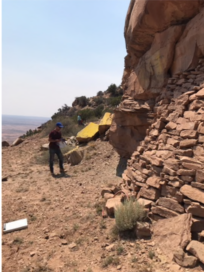
Photograph 2. An XRF survey in progress adjacent to a closed portal at Flag No.1 Mine.
