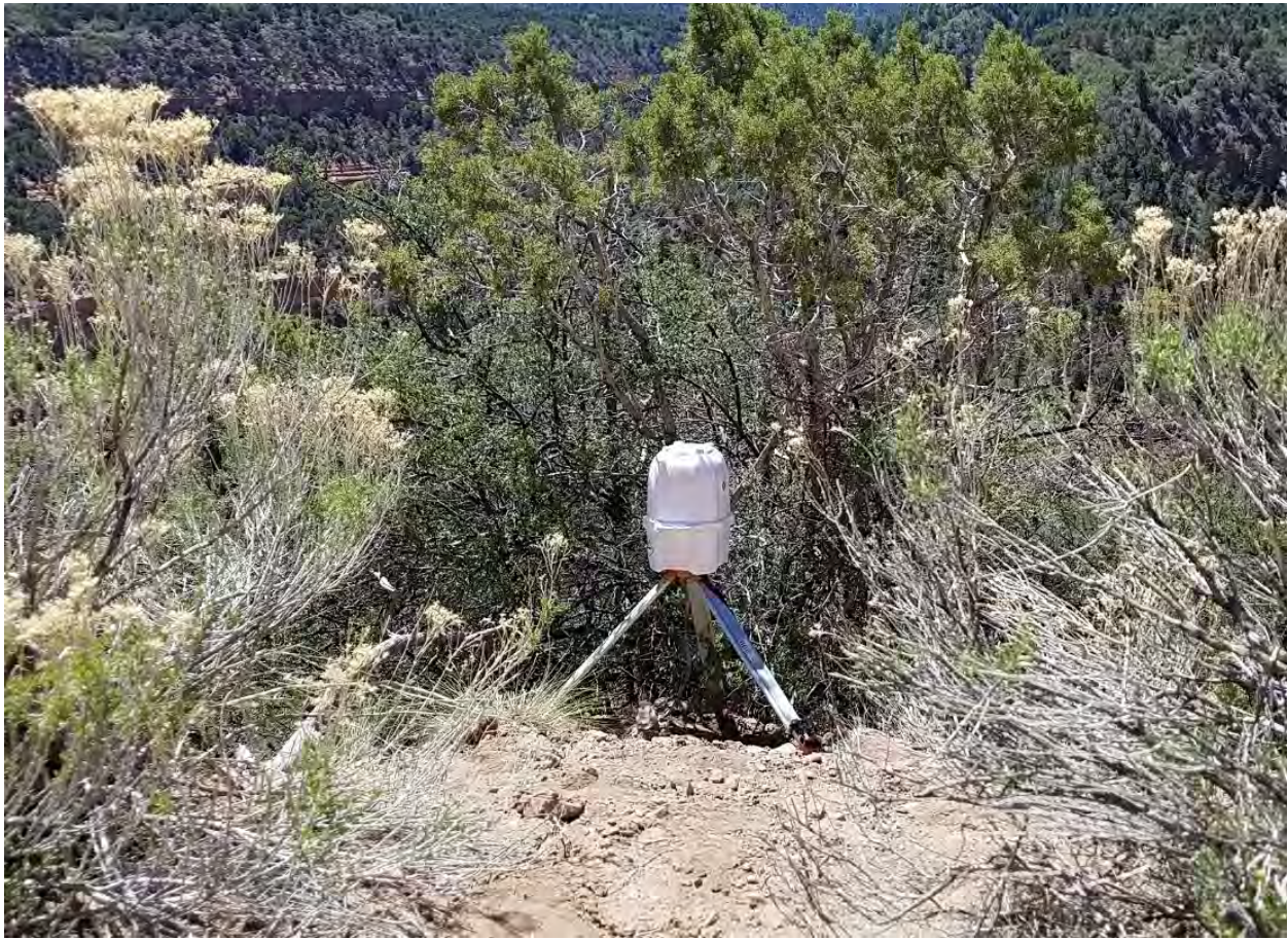
Figure 17. A High-Pressure Ionization Chamber
