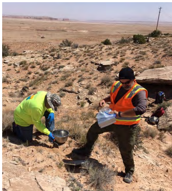
Figure 5. Field Crew Collecting Background Soil Samples at BSA-3
