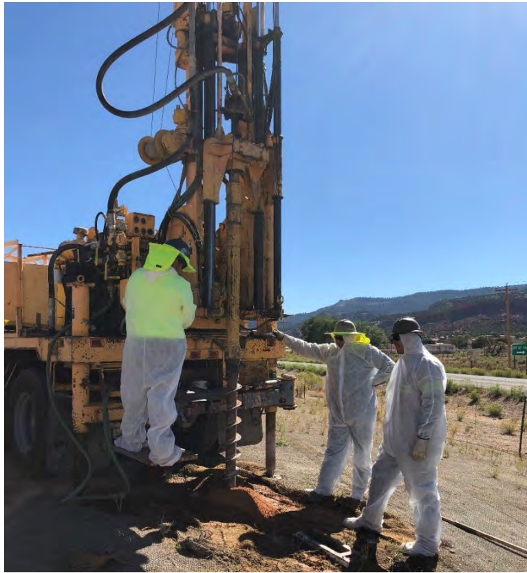
Figure 18. The Larger CME-75 Truck-Mounted Drill Rig
