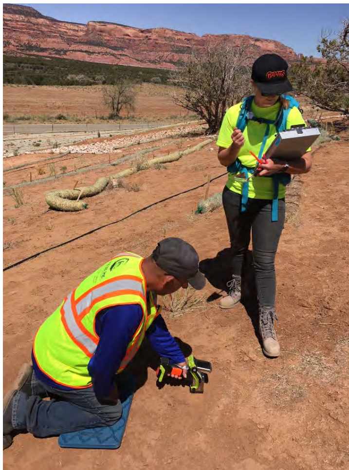
Figure 2. Field Team Performing XRF Survey at Subarea Group C
