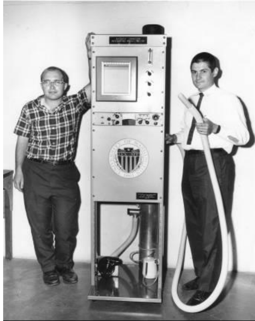
Norm Ahlquist and Bob Charlson with an early integrating nephelometer. UW Photo by William Eng, circa 1966
