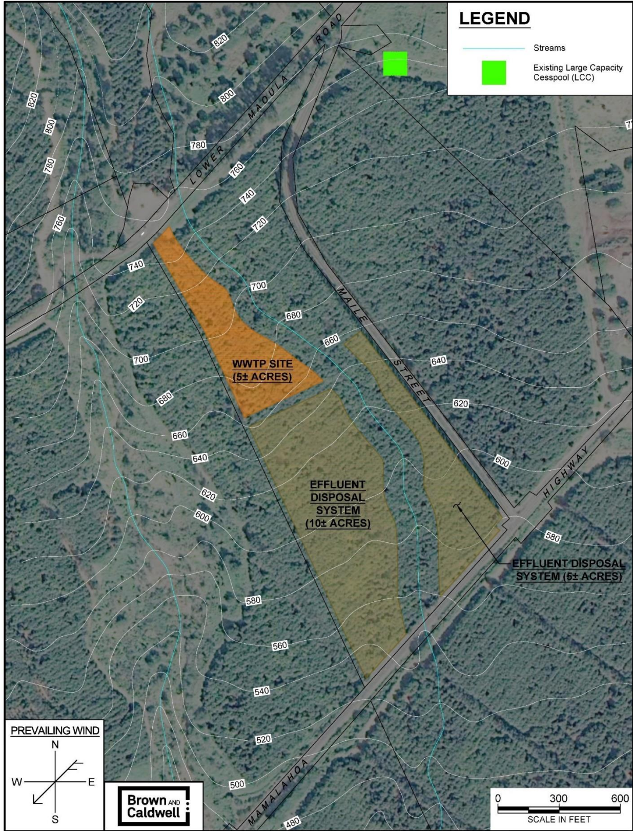
Figure 2.7. Site 8 Alternative – Preliminary Site Plan for New Wastewater Treatment and Disposal Facility
