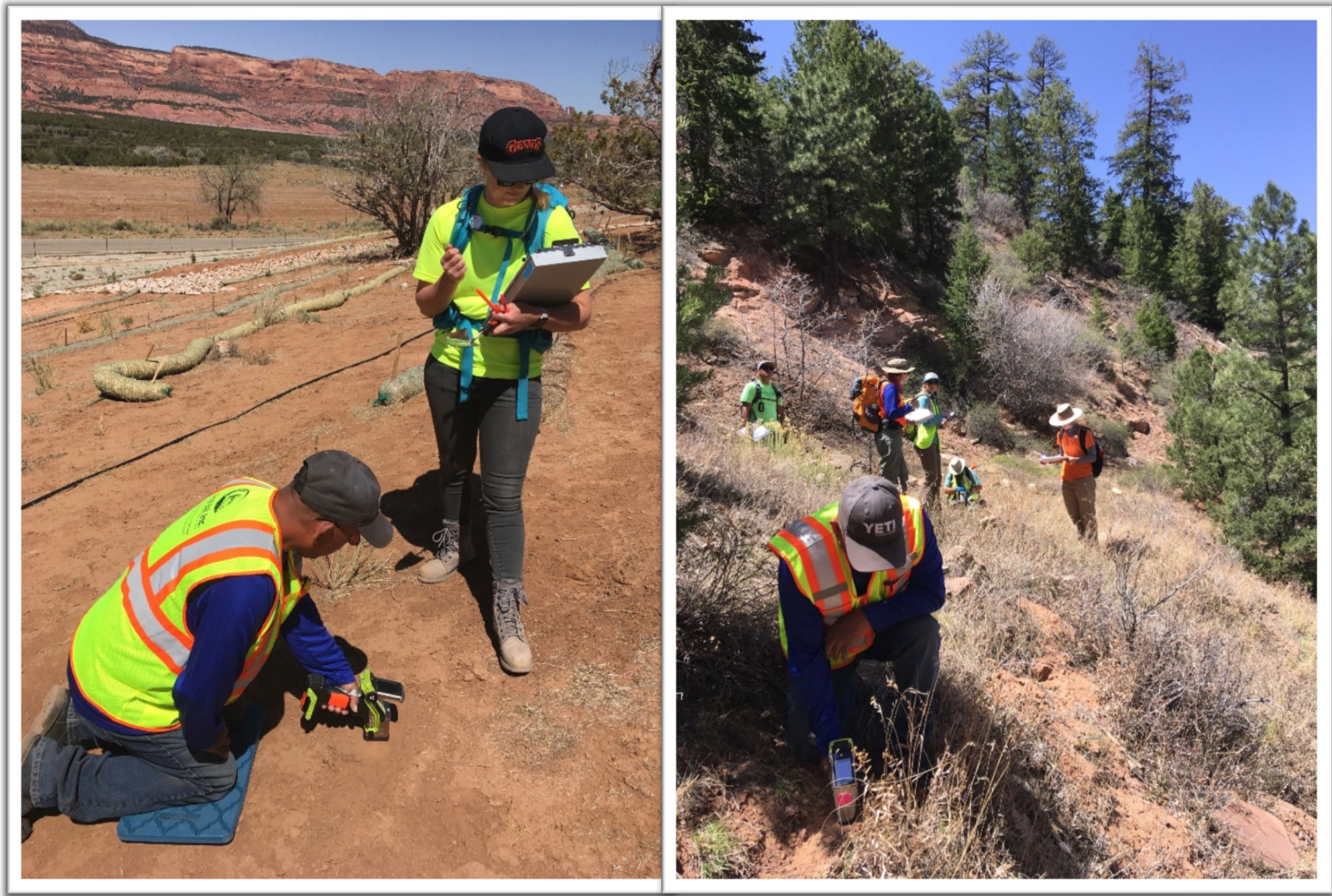
Figure B-8. Field Staff Taking In Situ XRF Measurements
