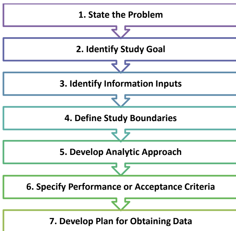
Figure F.2. Overview of a DQO process
