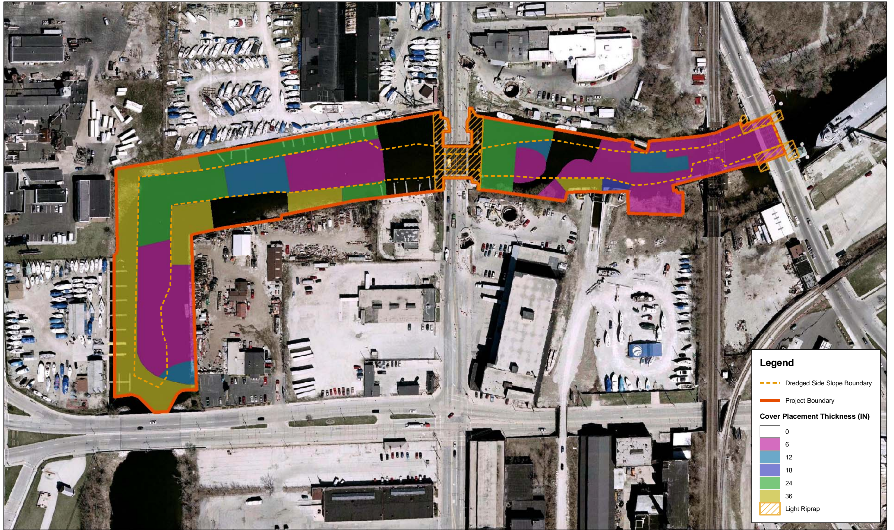
Figure 3-2 Sand Cover and Riprap Placement Kinnickinnick River Remedial Action Report Milwaukee, WI
