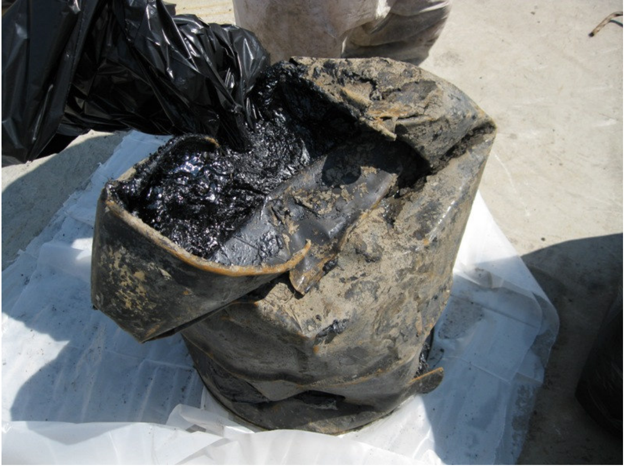
Drum of tar encountered during dredging in RMU1
