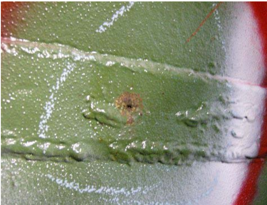
Flaw 347 through hole in strap
