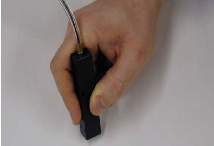
Above: The Hawkeye Pencil Probe used for testing all welds in tank # 2. Below: A TesTex crewmember using the Hawkeye a weld from one of the baskets.
