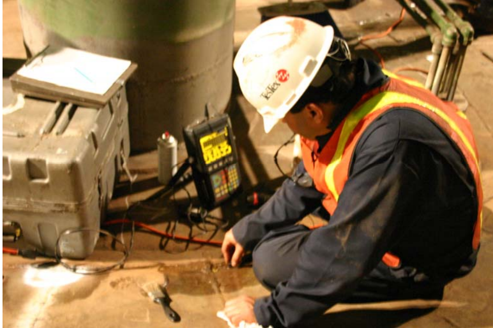
Photograph 1 – NDE technician/examiner performing angle beam UT measurements/examination of the intersection of the lower dome plates and the bottom plates.
