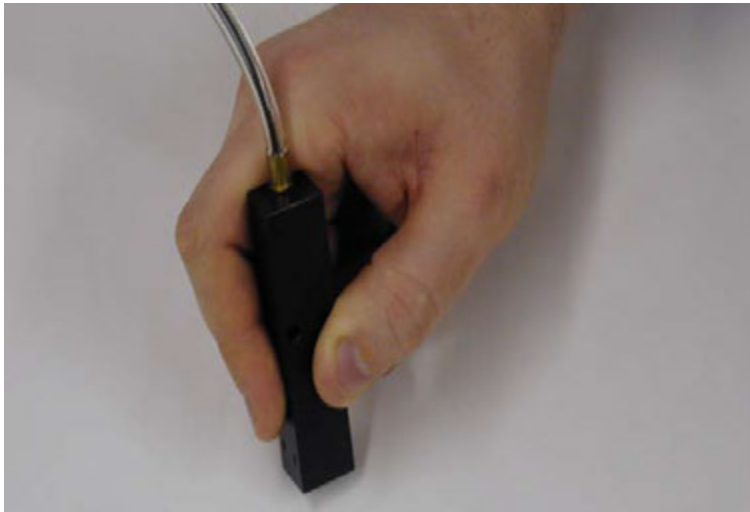
The Hawkeye Pencil Probe used for testing the welds of the floor, course 1, course 2, barrel, extension, and expansion of Tank #15.
