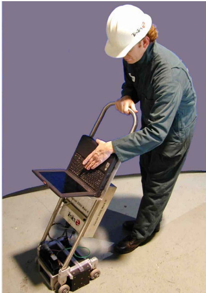
The Falcon Mark II 32 channel electromagnetic floor scanner used to scan the majority of the floor area in tank #15.
