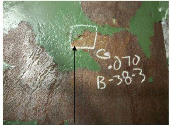
B-P38-4 GOUGE REPAIR
