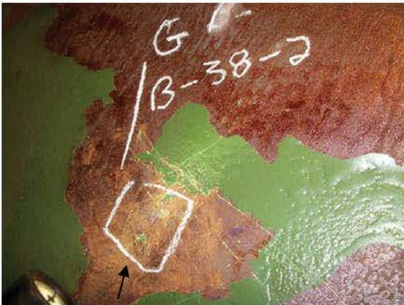
B-P38-3 GOUGE REPAIR
