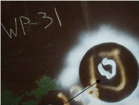
C-P16-1 PIT REPAIR
