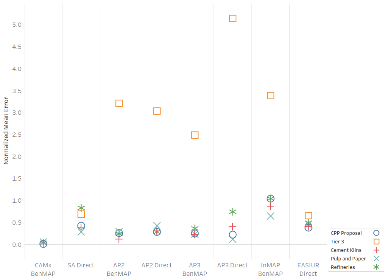
EXHIBIT 3-7. NORMALIZED MEAN ERROR OF REGIONAL ESTIMATES BY MODEL, COMPARED AGAINST CMAQ ESTIMATES
