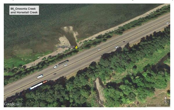
The upstream extent was set at the I-84 overpass, 0.03 miles (0.05 km) upstream. Due to the creek being a low flow tributary, stream depth likely limits CWR use upstream of this point.
