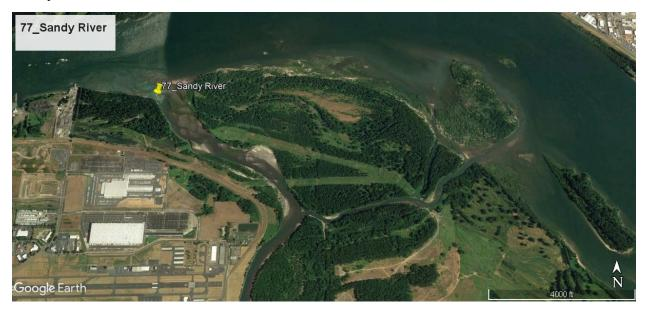
The upstream extent was set where the river channel in the delta was at maximum depth of 0.8 meter based on a site visit conducted on 8/30/18, 0.19 miles (0.3 km) upstream of the interface of the Sandy River and the Columbia River. The lower section of the Sandy River is a shallow delta and is tidally influenced.
