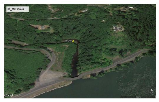
The upstream extent was set at the first riffle, 0.15 miles (0.24 km) upstream. Stream gradient increases above this point, based on field observations. The upstream extent does not appear to be tidally influenced.
