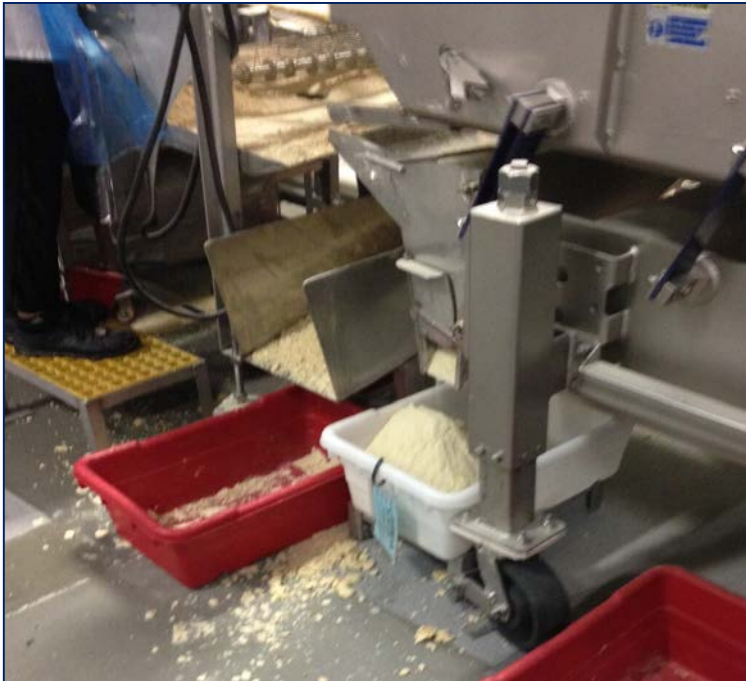
Batter coating loss from vibrational alignment
