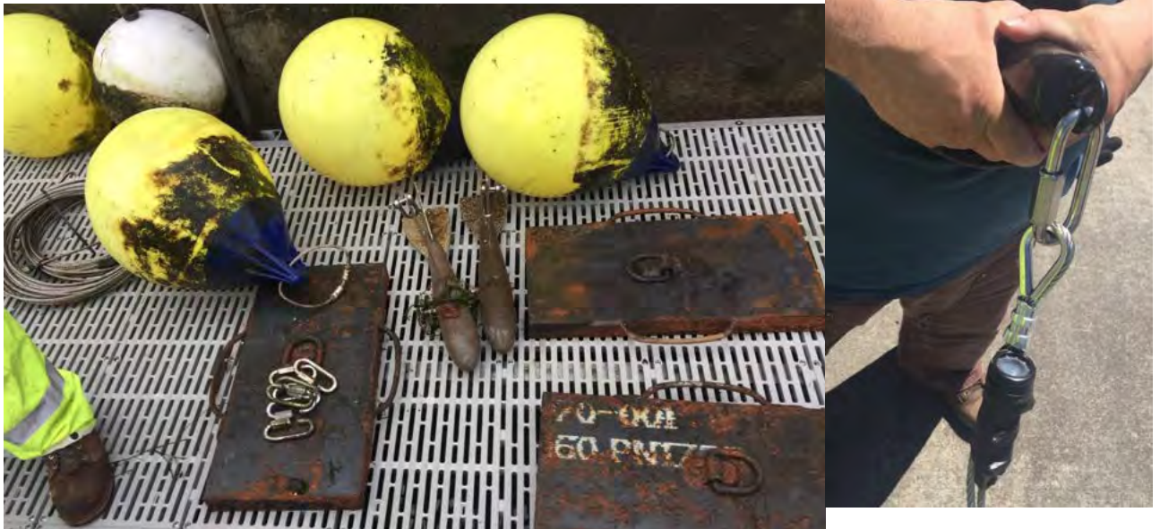
Figure 3-2. Equipment for the Floating Temperature Strings, including Yellow Buoys, Fish Weights (30-lb), Steel Anchor Plates (170-lb), and Mushroom Weight (30-lb) for the Wall Mounted Strings, with Cable and Data Logger Attached (on right).
