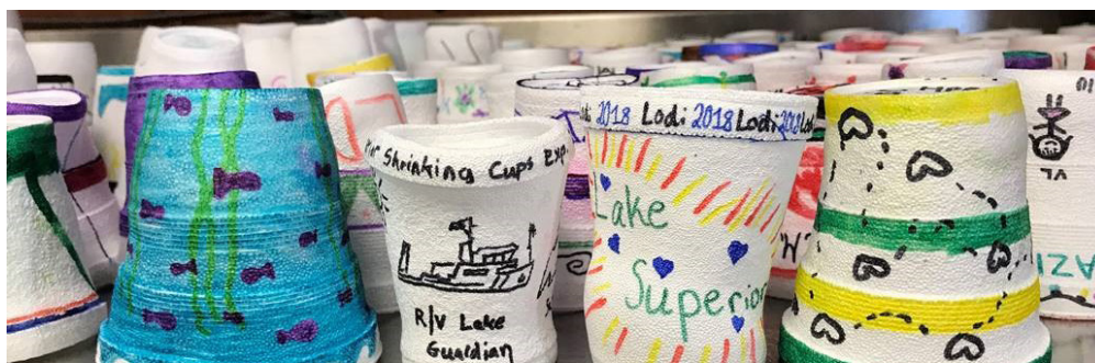
Polystyrene cups were crushed under pressure at the bottom of Lake Superior
