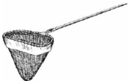
Figure 6.3 D-frame net (500 µm mesh) used for collecting benthic macroinvertebrates.
