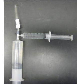
Figure 5.6 Glass vial connected to 3-way stopcock
