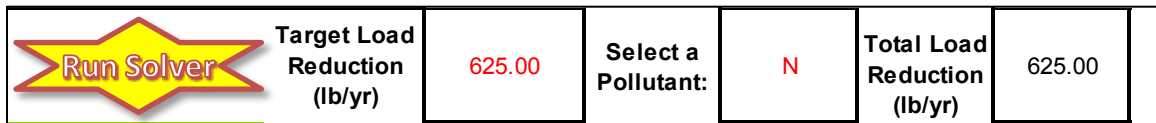
Figure U11. Run Solver button to run optimization scenario and the inputs for target load reduction and pollutant of concern.
