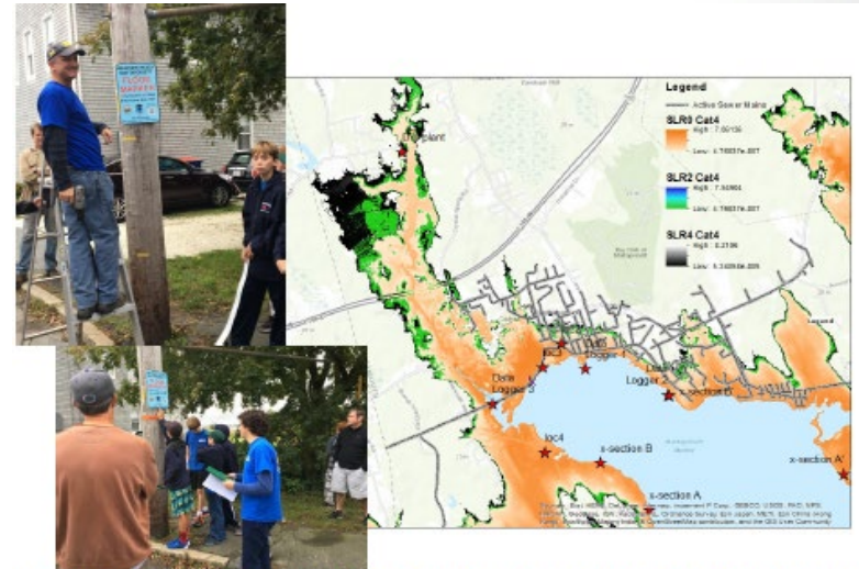
Figure 2. SLOSH modeling results of storm surge inundation for category 4 hurricane and 4-ft sea level rise scenario, with impacts to the wastewater collection and transfer systems. Citizens were engaged in historical flood level identification as a part of the citizen science project.
