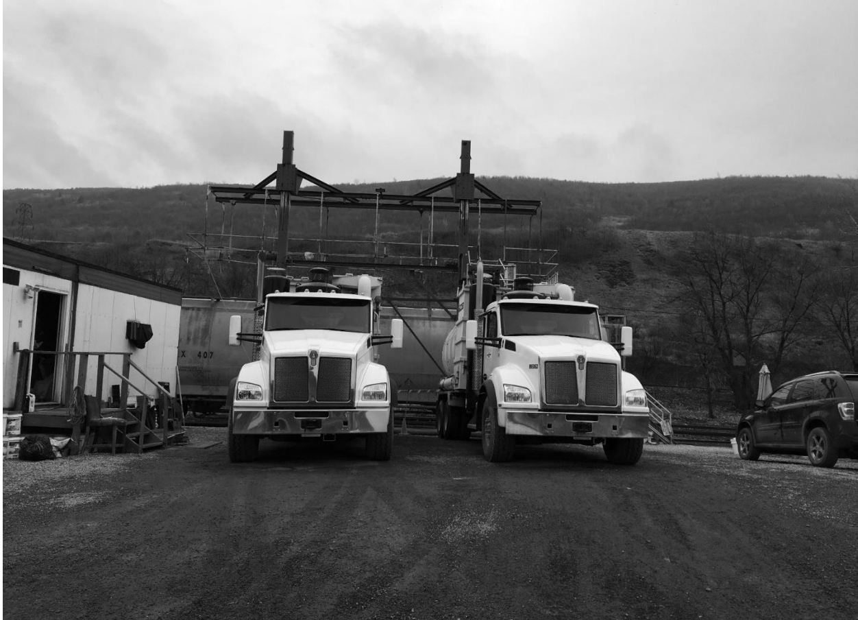
Figure 5 - Railcar Vacuum Unloading (Vac-Rack)
