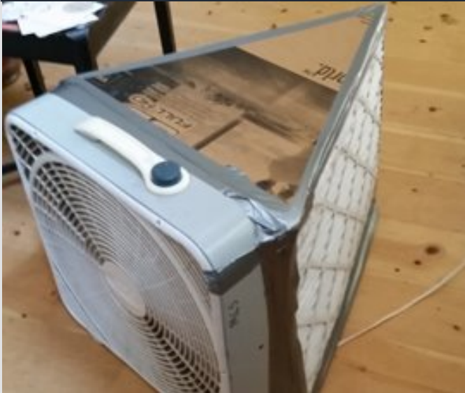
DIY Air Cleaner, Deluxe Model. Photo Credit: Dave Conway, Mariposa County APCD
