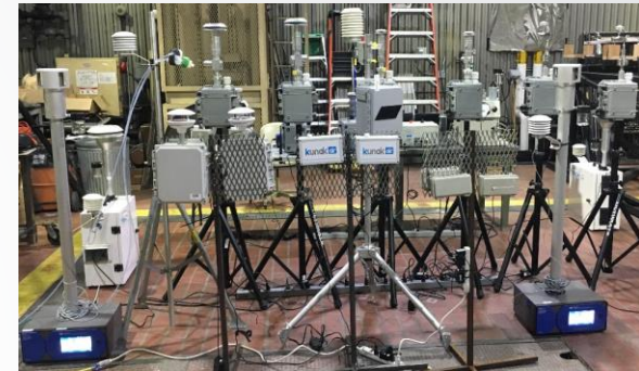
Sensor pod evaluation at USFS Missoula Fire Science Lab
