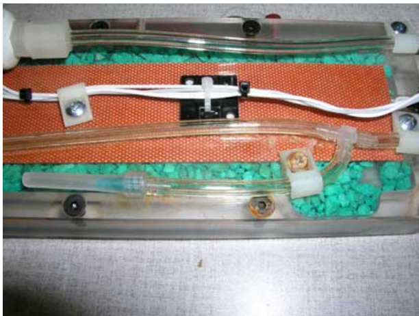
Crushed scrubber tubing
