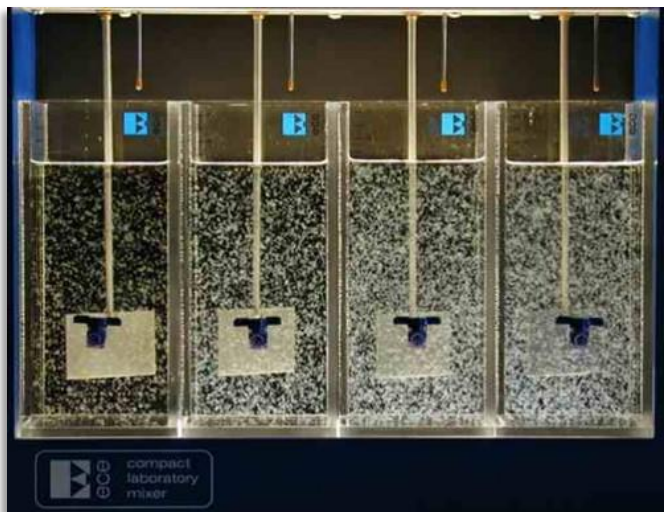
During jar testing, coagulant concentrations can be compared to determine the coagulant dose that results in the greatest removal of DBP precursors.
