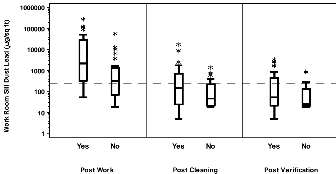
Figure D2.9a. Box Plots of Sill Dust Lead Loading in the Work Room by Stage and Restricted Job
