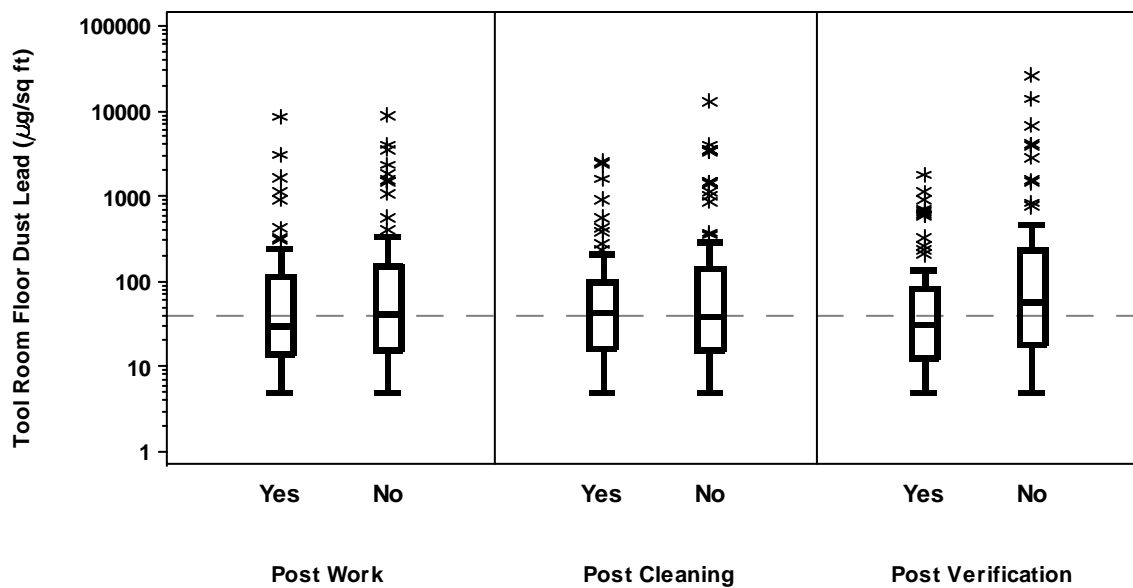
Figure C2.6b. Box Plots of Floor Dust Lead Loading in the Tool Room by Stage and Rule Plastic Use
