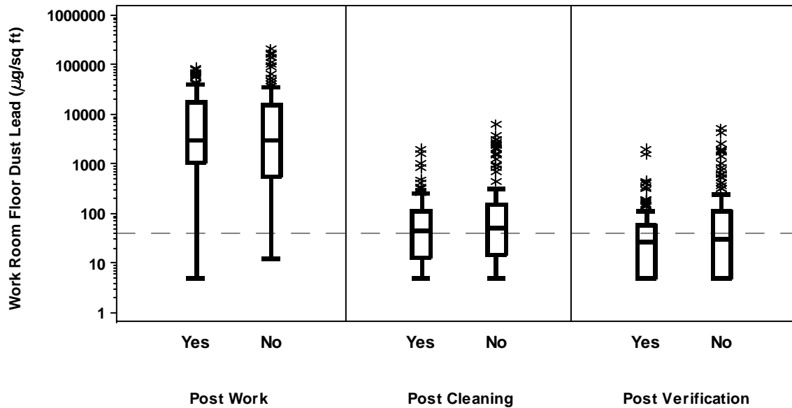
Figure C2.6a. Box Plots of Floor Dust Lead Loading in the Work Room by Stage and Rule Plastic Use
