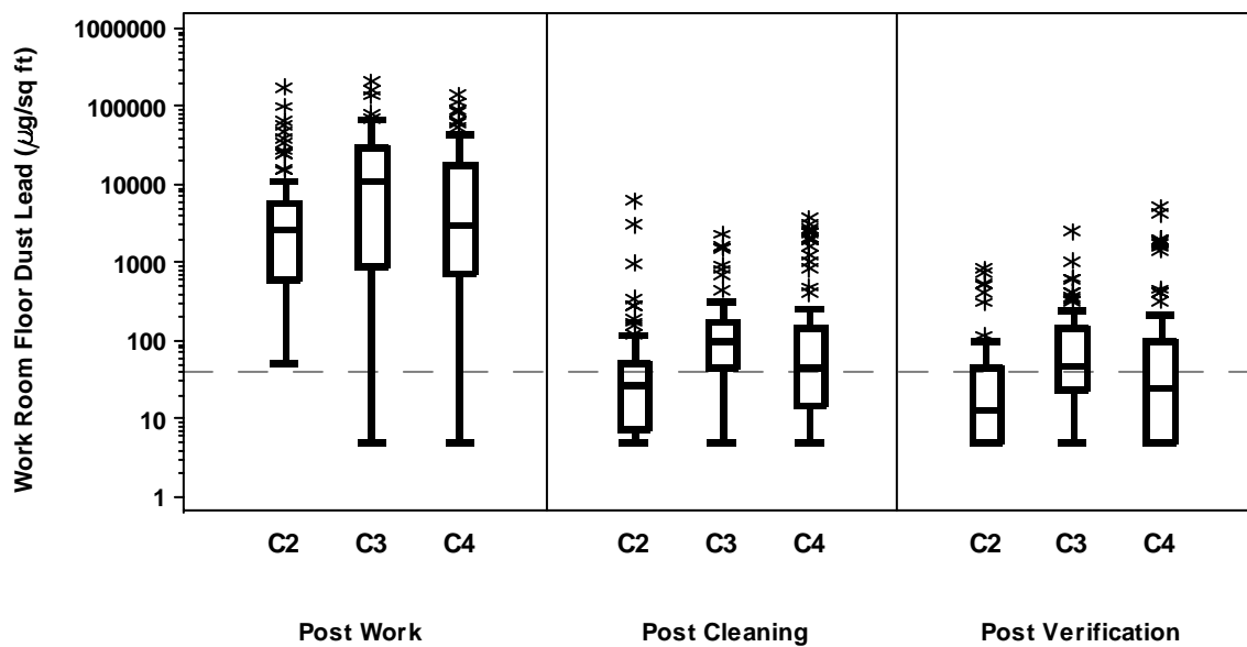
Figure C2.4a. Box Plots of Floor Dust Lead Loading in the Work Room by Stage and Contractor
