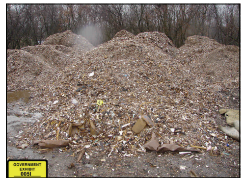
Piles of illegally dumped asbestos-contaminated debris at the site.
