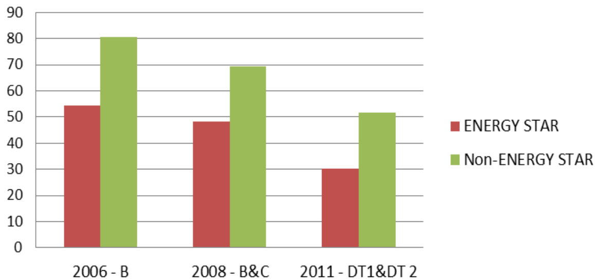
Desktop Idle (W) Over Time - Based on Business Desktop in ES Data Sets
