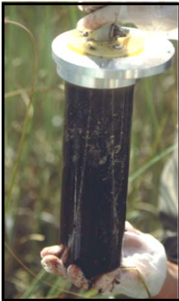
Figure 14. Soil cores were collected at each of the marsh sites and analyzed for mercury, nutrients, and other constituents.
