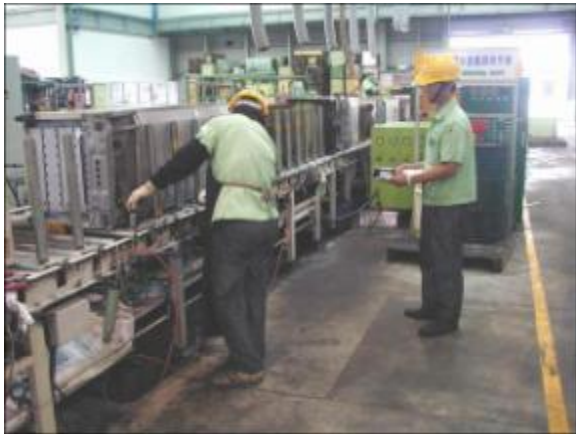
Extracting the refrigerant 冷媒抽取
