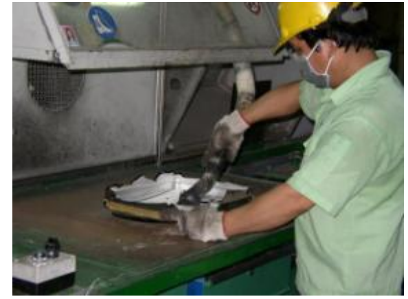
Fluorescent powder Collect 螢光粉吸取
