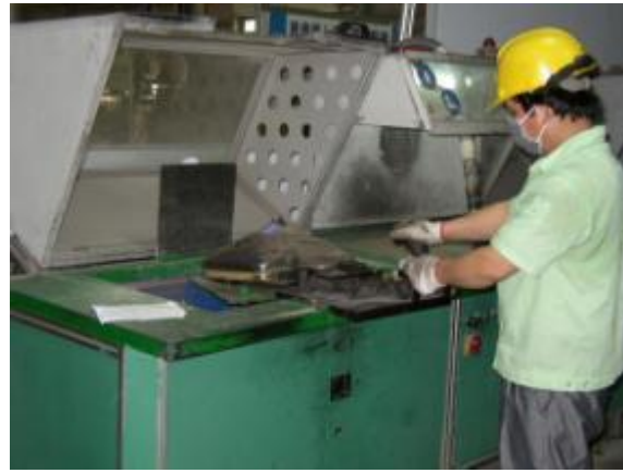
Cutting the CRT tube 映像管切割
