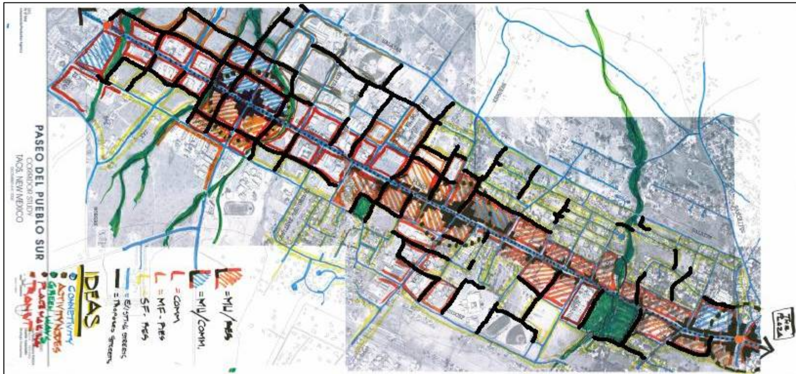
Figure 12: Map with potential new street connections highlighted in black. New streets are conceptual only; this map illustrates small, strategic street connections that could help traffic to circulate more easily, not specific places where the team is recommending new streets be built. (Thick lines are used to make the potential streets easier to see; they are not intended to suggest any specific street width.)
