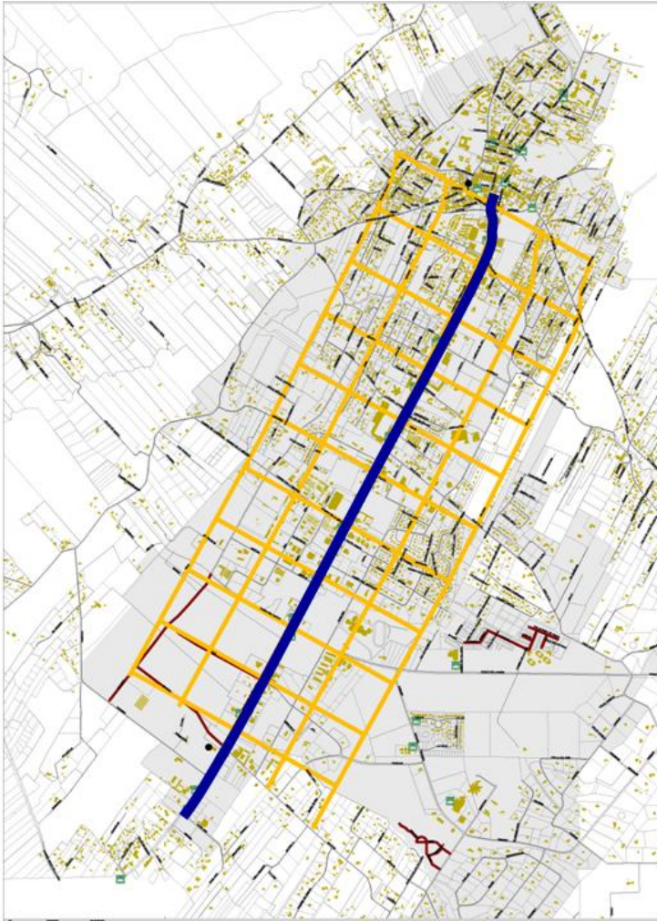
Figure 10: A conceptual street grid, with arterials at 1-mile intervals
