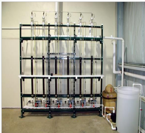
Anaerobic treatment column studies at EPA pilot plant.
