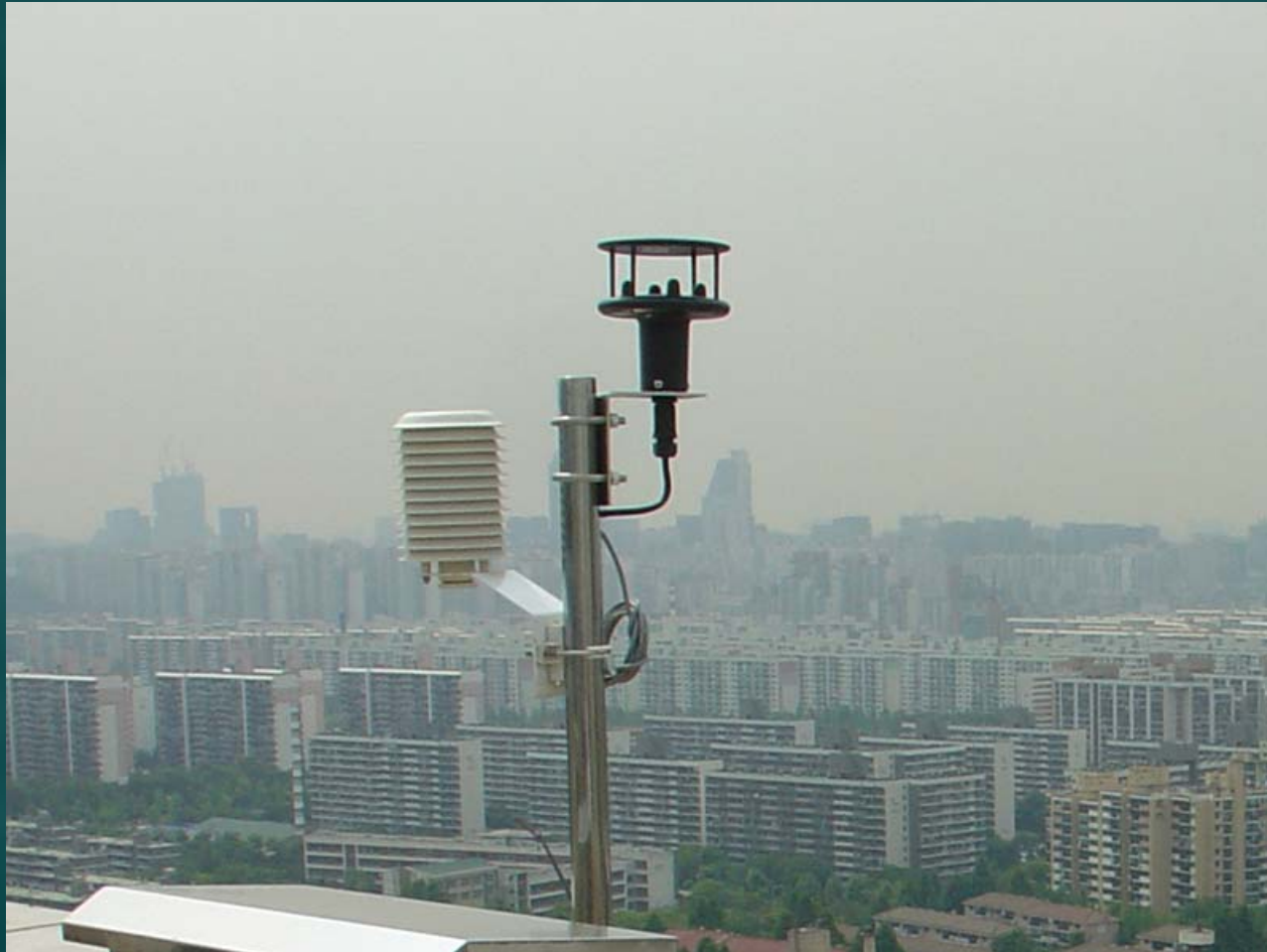
Example of Sonic Anemometer & Solar Radiation Shield
