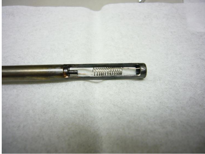
Figure 5. Pyroprobe Pt filament
