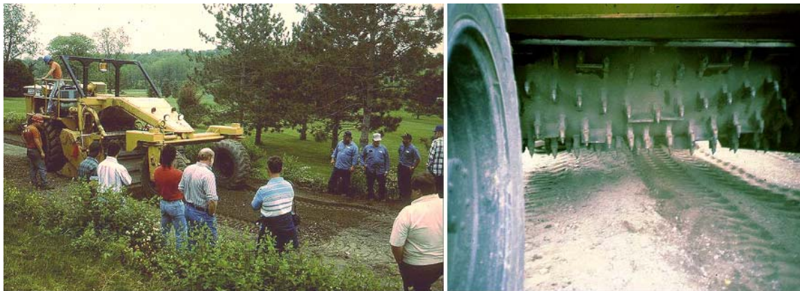
7-12 The “reclaimer” has a down-cutting drum with carbide teeth.
