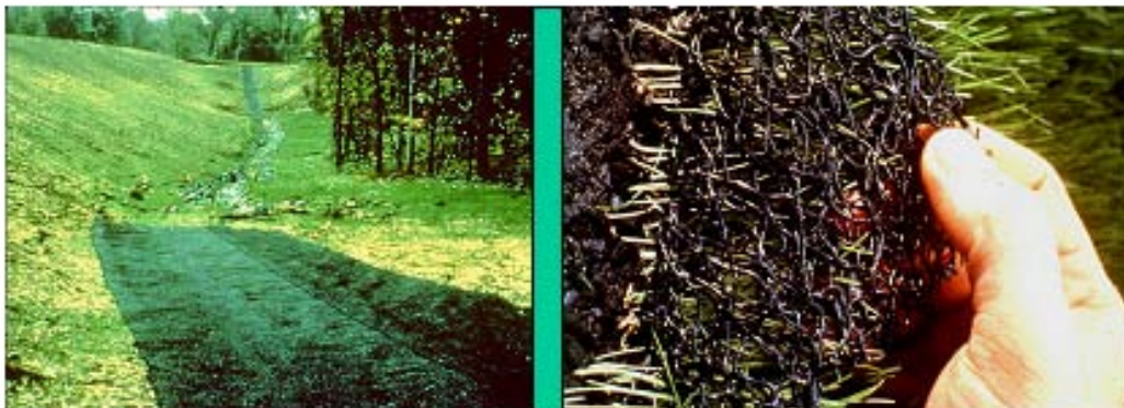
5-15 Many geosynthetic products are available for erosion prevention.
