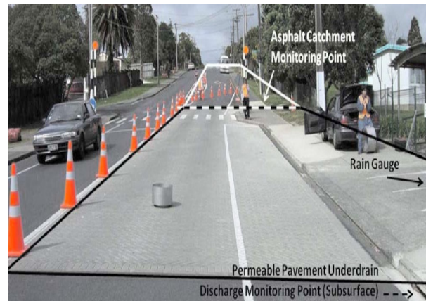
Figure 13. Permeable Concrete Paver Block Test Site
