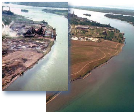
Figure 1. These pictures of the Cherry Farm/Roblin Steel federal Superfund site show the difference between the actively polluting site in 1960 (left) and the post-remediation site in 2001 (right).
