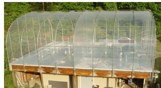
UNC 274-m 3 Dual Outdoor Smog Chamber
