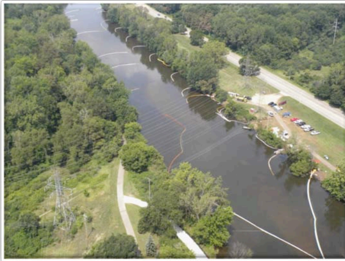
Figure 16 – Containment Boom in Cascade Configuration in Division D (8/7/2010)
