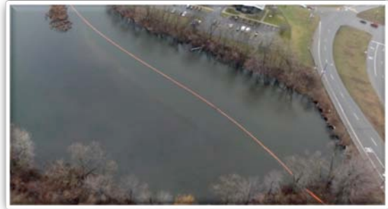
Figure 54 – Chevron Boom Upstream of Ceresco Dam (10/11/2011)
