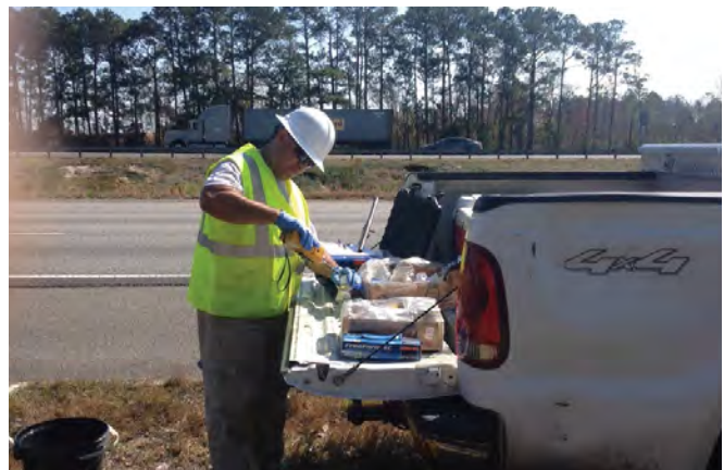
At the scene of a diesel spill on a highway in Jacksonville, Florida, Ruben Rodriguez is testing a soil sample, using a glass jar and a photoionization detector.
