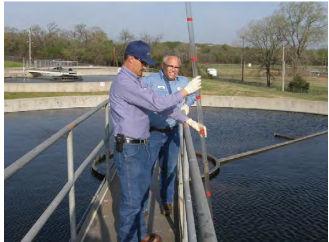
Graduates Larry Forsyth and James Whalen measure sludge depth in a water clarifier on the job at the Edmond Coffee Creek Wastewater Treatment Plant.
