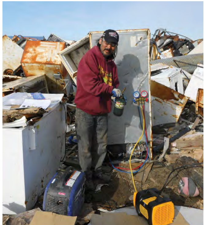
Basil Lake uses the required specialized equipment to remove Freon from a refrigerator at a dumpsite in Hooper Bay.
