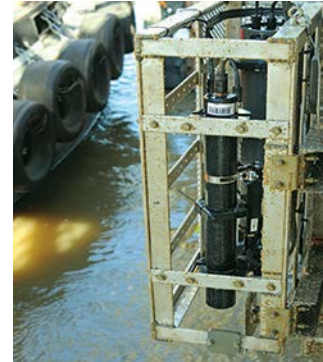
Continuous ultraviolet nitrate sensors and other water quality instruments deployed in the Mississippi River allow for a better understanding of nitrogen dynamics at the rates in which changes occur.
