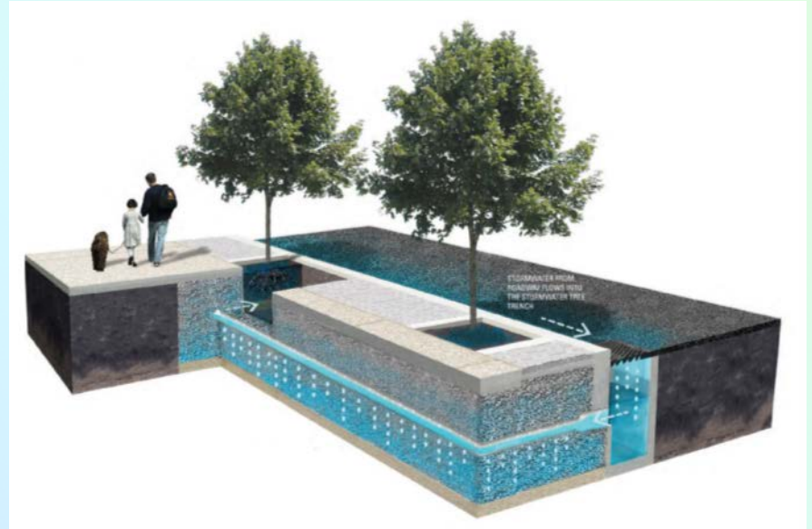
Stormwater tree trench
