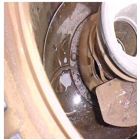
Damaged seal in poor condition
