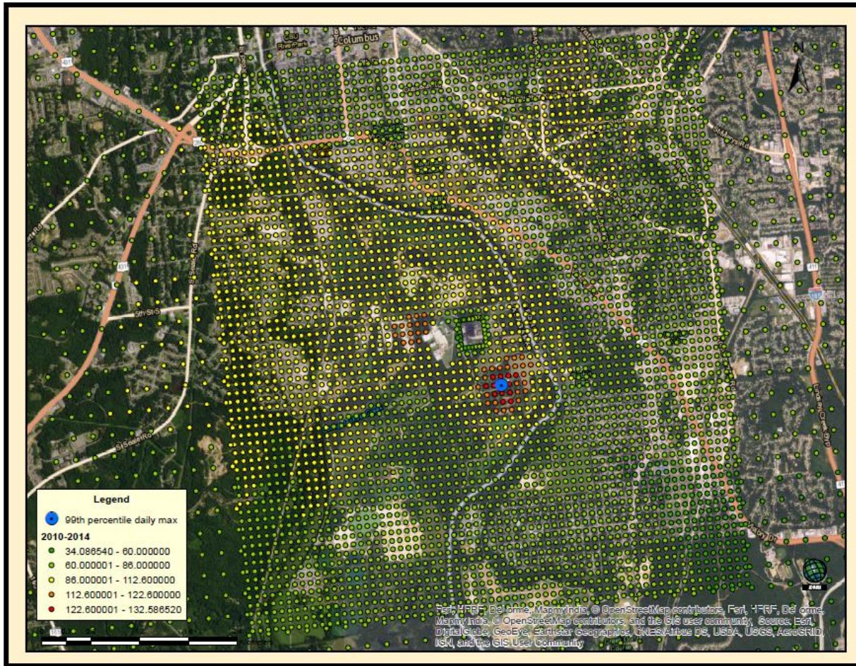
Figure 60. Maximum Predicted 99 th Percentile Daily Maximum 1-Hour SO 2 Concentrations Averaged Over Three Years for the Area of Analysis for the Russell County Area
