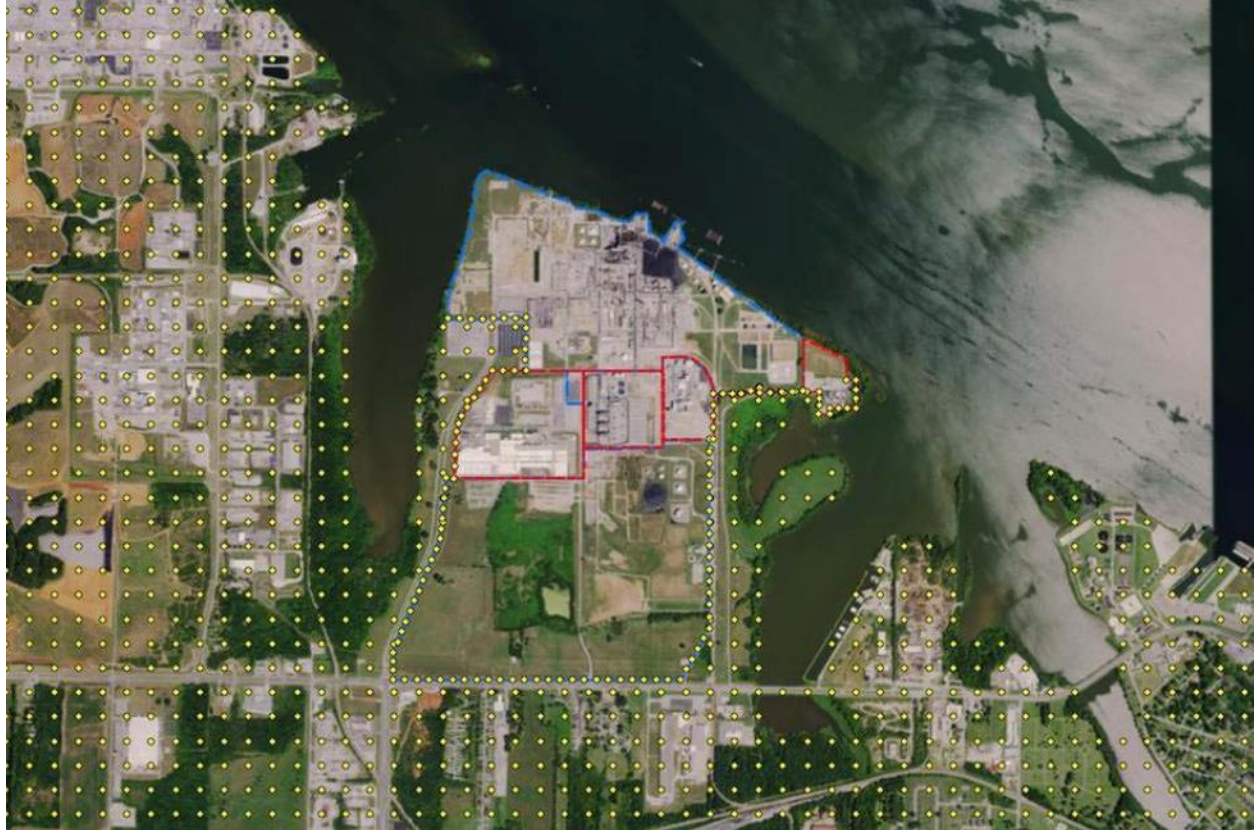
Figure 37. Modified Receptor Grid with Receptors over Roads and Parking Areas around the Ascend Facility. Source: “Air Dispersion Modeling for Evaluating Compliance with the 1-Hour SO 2 National Ambient Air Quality Standard at the Ascend Performance Materials Facility in Decatur, Alabama” prepared for Alabama, December 2016
