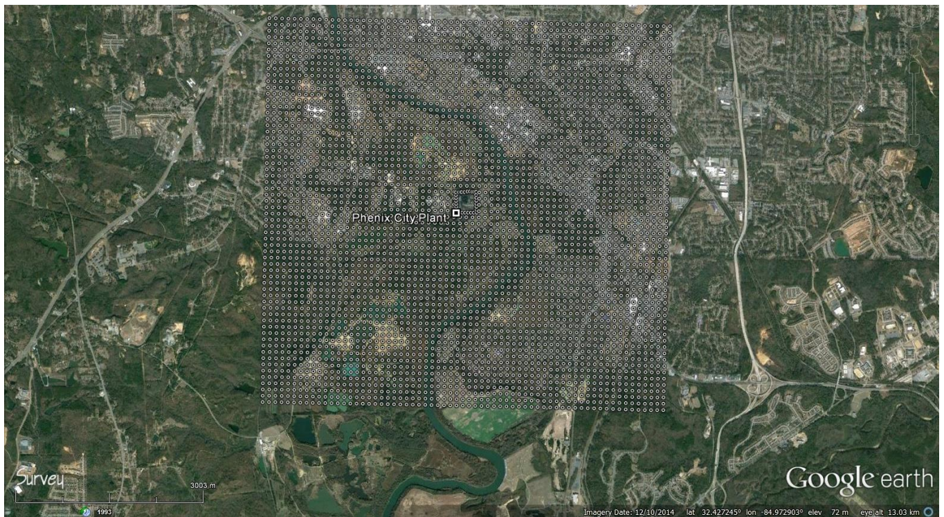
Figure 53. Tight Receptor Grid for the Russell County Area. Source: "Air Dispersion Modeling Report Air Quality 1-Hr SO 2 Compliance Demonstration Phenix City Plant Continental Carbon Company Russell County Phenix City, Alabama" prepared for Alabama, December 2016.
