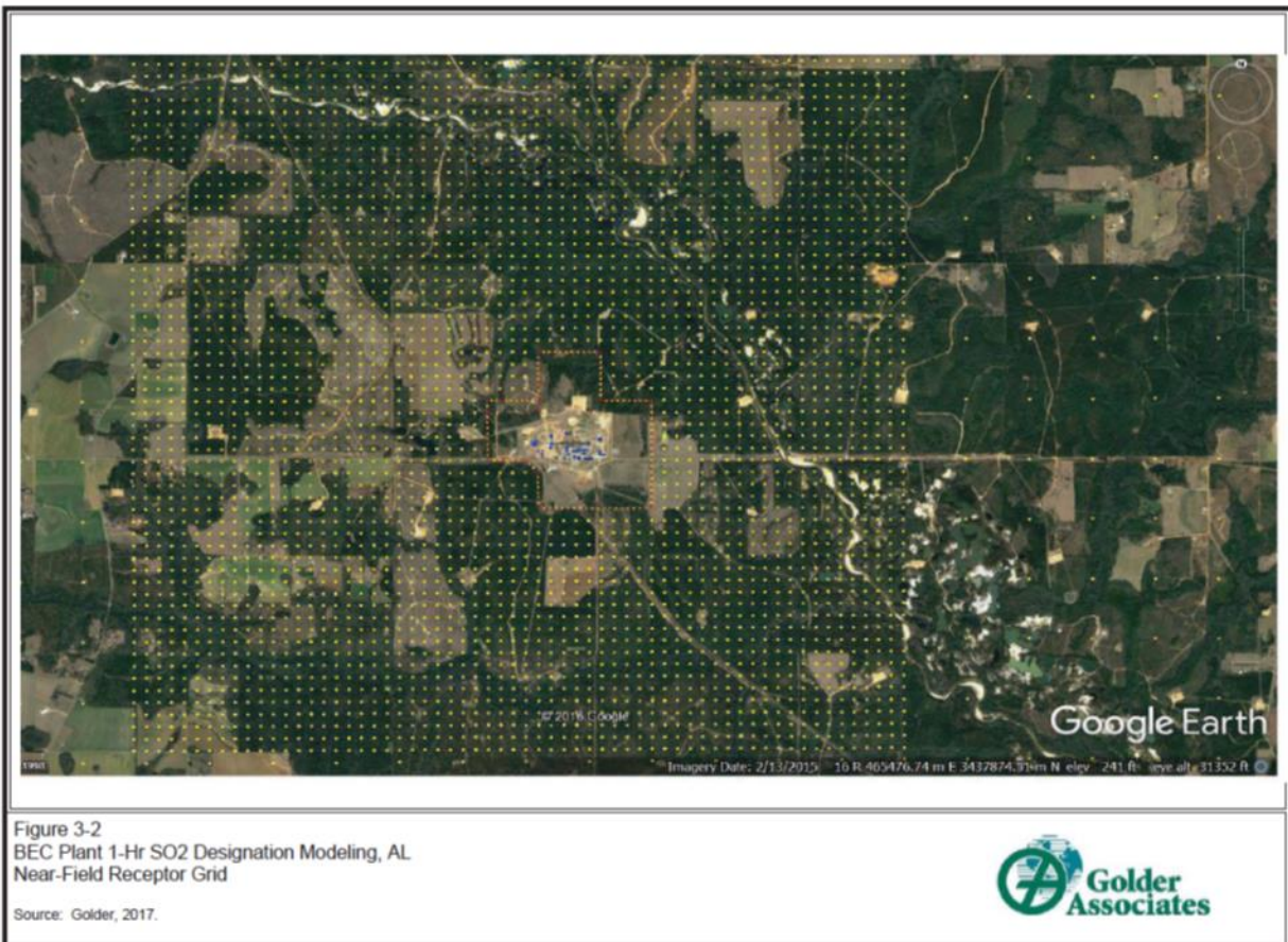
Figure 20. Near-Field Receptor Grid for the Escambia County Area. Source: “Air Dispersion Modeling for 1-Hour Average SO 2 NAAQS Area Designation Big Escambia Creek Plant, Escambia County, Alabama” prepared for Alabama, January 2017.
