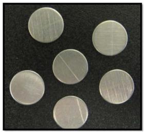
Fig. 2: Examples of typical unacceptable 430 SS carriers.
