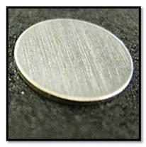
Fig. 1: Examples of typical acceptable 430 SS carriers.
