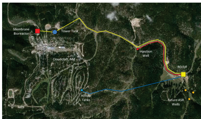
Figure A.4-3. PRe water pipeline from WWTP to water treatment facility (Courtesy of Eddie Livingston from Livingston Associates)
