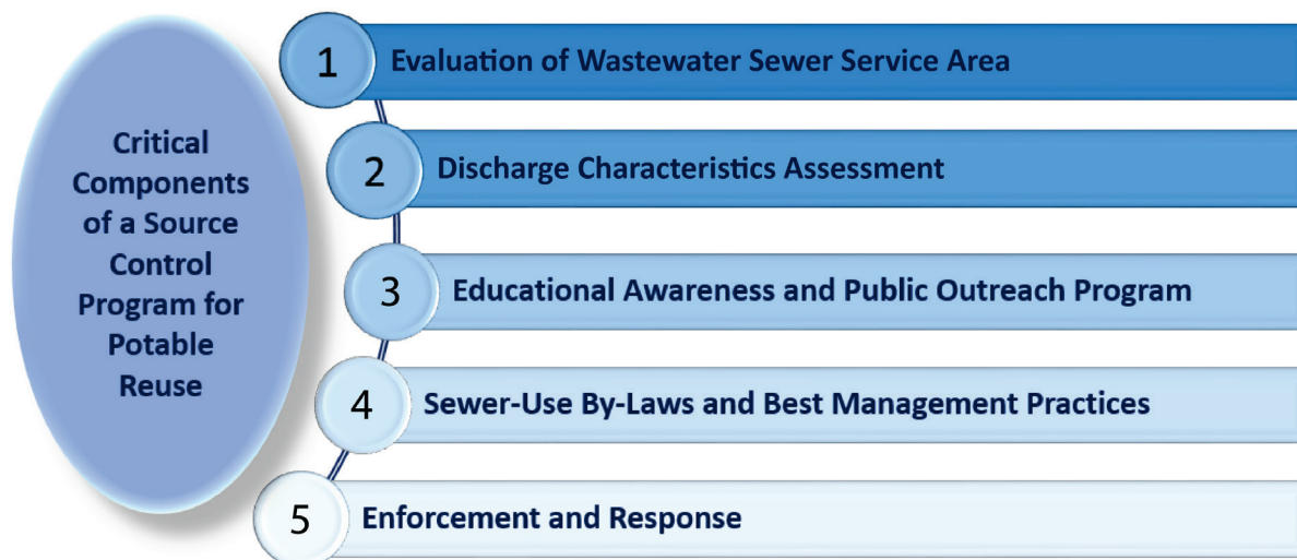
Figure 8-2. Critical components of a source control program for potable reuse
