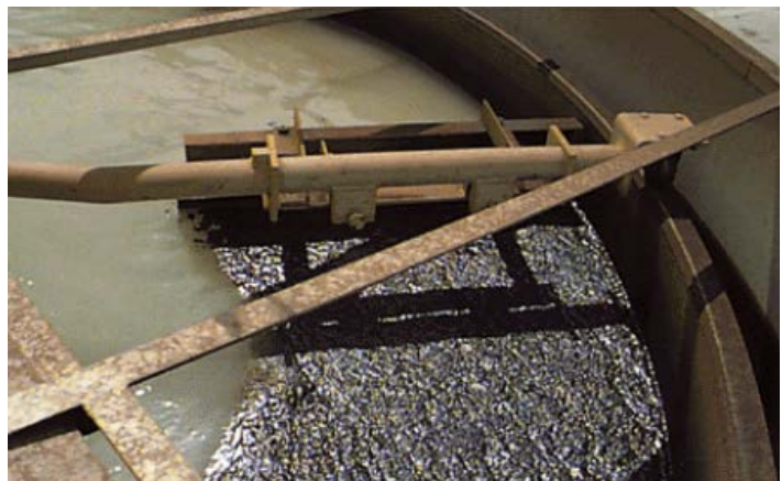
Contaminants in a dissolved air flotation tank at Visalia Pole Yard (Walter, 1998)
