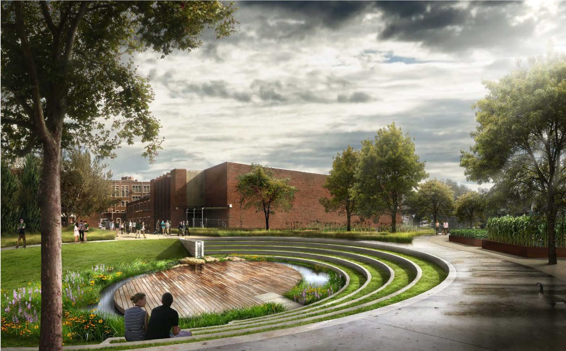
Figure 30. The design option includes a recessed amphitheater to capture and detain water from the building and parking areas, and constructed wetlands to collect and infiltrate stormwater from adjacent streets.
