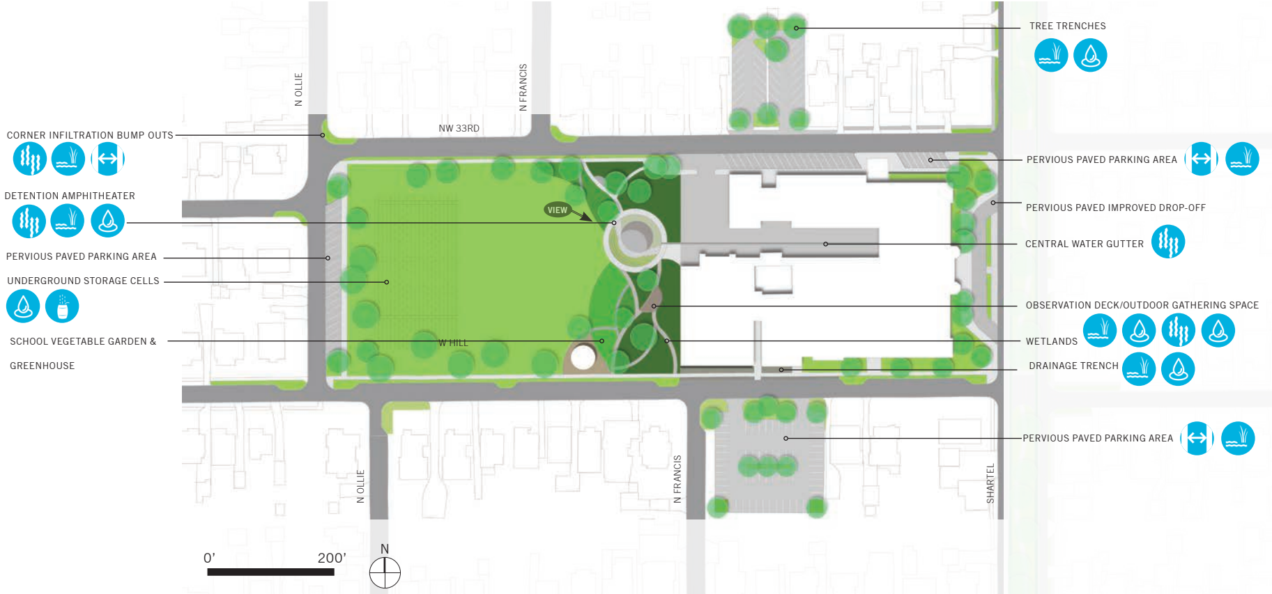
Figure 27. The design option for Harding integrates outdoor learning areas with stormwater management infrastructure, and introduces pervious paving to parking areas. The Edison Green Campus pervious parking lot image on page 33 illustrates a similar green infrastructure design for student and faculty parking lots.
