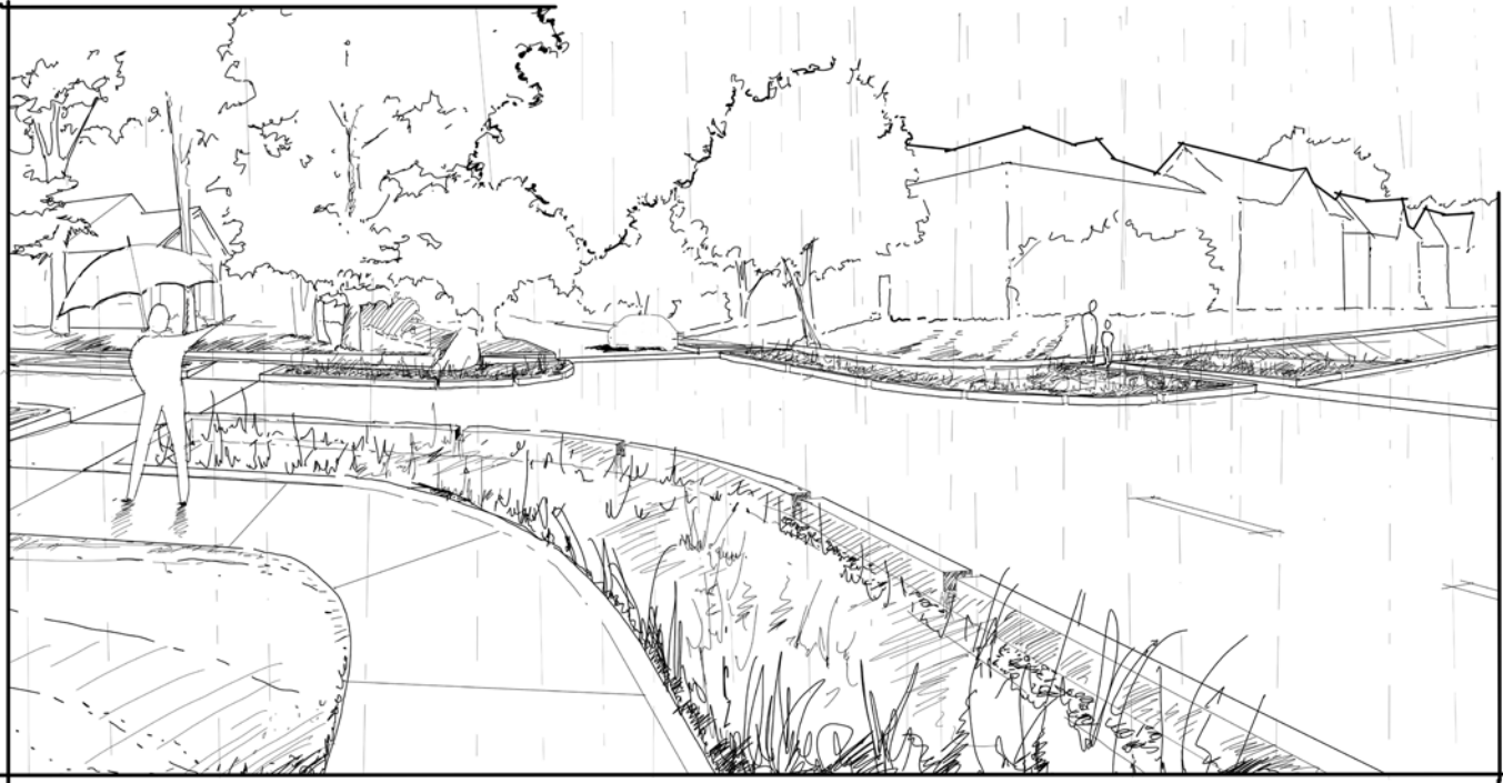
Figure 41. Sketch of rain garden bump-outs integrated into new street design at Walker Avenue intersection.
