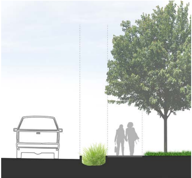
Figure 43. This section illustrates how stormwater is infiltrated in vegetated bioswales between the street and sidewalk.
