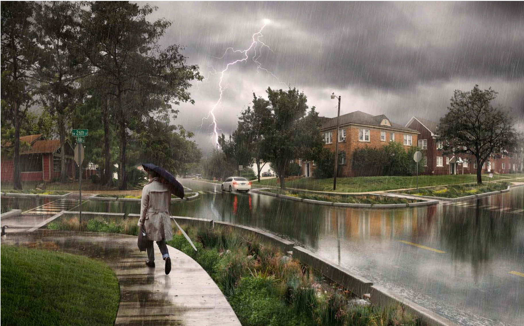
Figure 45. Rain garden bump-outs slow traffic and infiltrate stormwater. Continuous sidewalks and well-marked crosswalks improve walkability and pedestrian safety.
