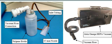
Figure 2. Modified Wet Vacuum from Dry Vacuum
