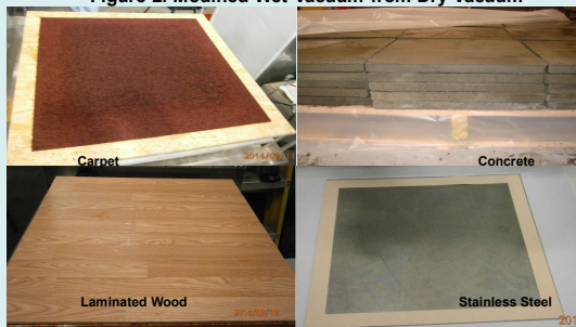
Figure 3. 28 x28 in Test Coupons
